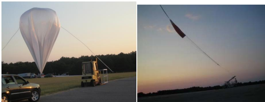
**Figure 23-1-2-2. Tiny Tim and the ARCADE 2 payload at launch. The parachute connecting the payload to the balloon is clearly visible.**
